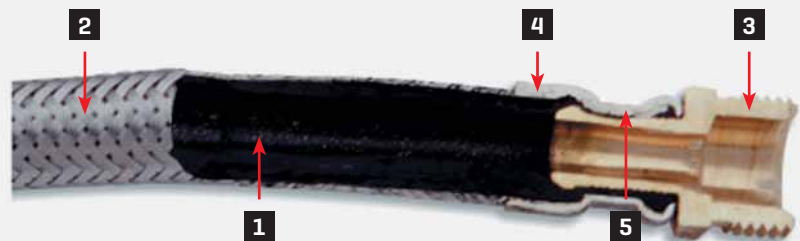
1: Innertube of either EPDM for water or Nitrile for fuel gas. 2: 304 stainless steel braid. 3: End fittings made from either DR brass, free machined brass or chromed steel. 4: 304 stainless steel ferrules. 5: Crimping.
