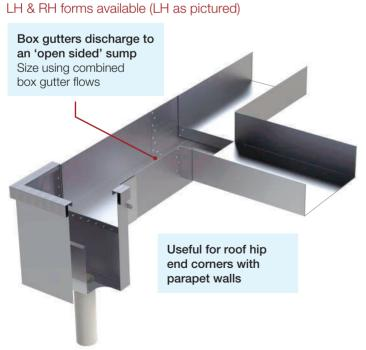
Allows 3 x box gutters to intersect and discharge to a single Dam Buster Rainhead. Size using combined box gutter flows.
